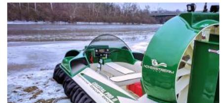
The composite hull with Kevlar reinforcement is strong and durable, yet lightweight. It's ready to work in saltwater operations and the harshest commercial conditions.
