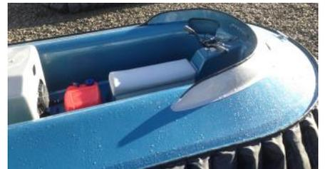
The Snapper II has a low seat with the driver in a kneeling position. This enhances the sporty feel of the machine... shift some of your weight to one knee or the other and the hovercraft will turn that direction.
